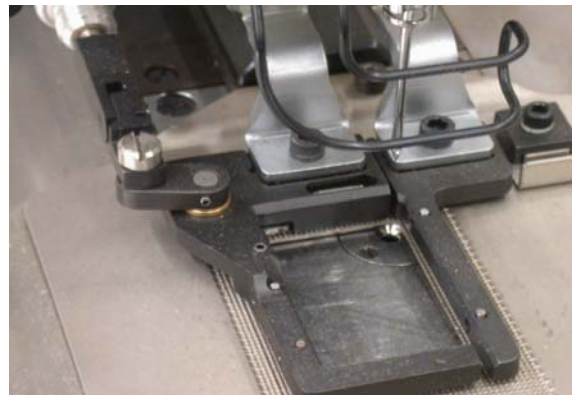
View of custom upper work clamp assembly with built in needle thread trimming knife
